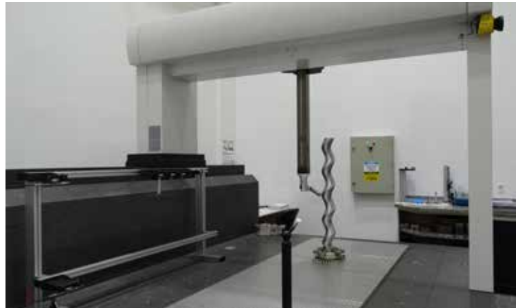
Precision measuring equipment is used to provide the right tolerances and best fit for pump components.
